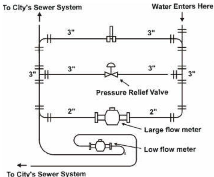
Figure 2: Metered Piping System Schematic (South Side)
