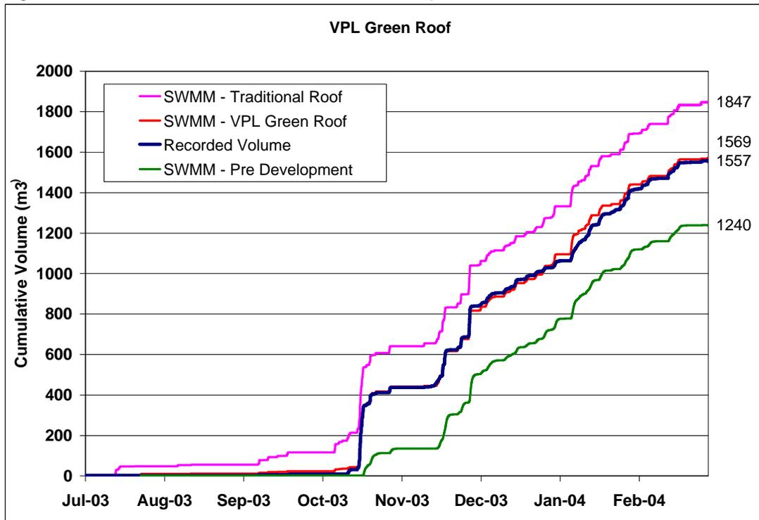
The results would indicate that the green roof at the VPL is significantly reducing the volume of runoff from when compared to a traditional torch-on membrane style roof.
