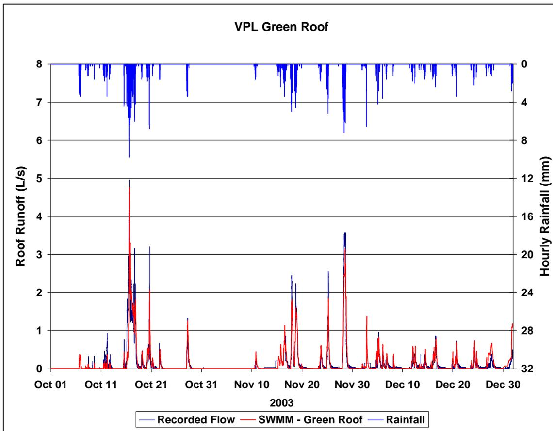
To create the traditional roof model, the calibrated model impervious area was increased to 100% to simulate a torch-on style roof. The natural condition’s model was developed using calibrated parameters for undisturbed, forested areas based on previous work.
