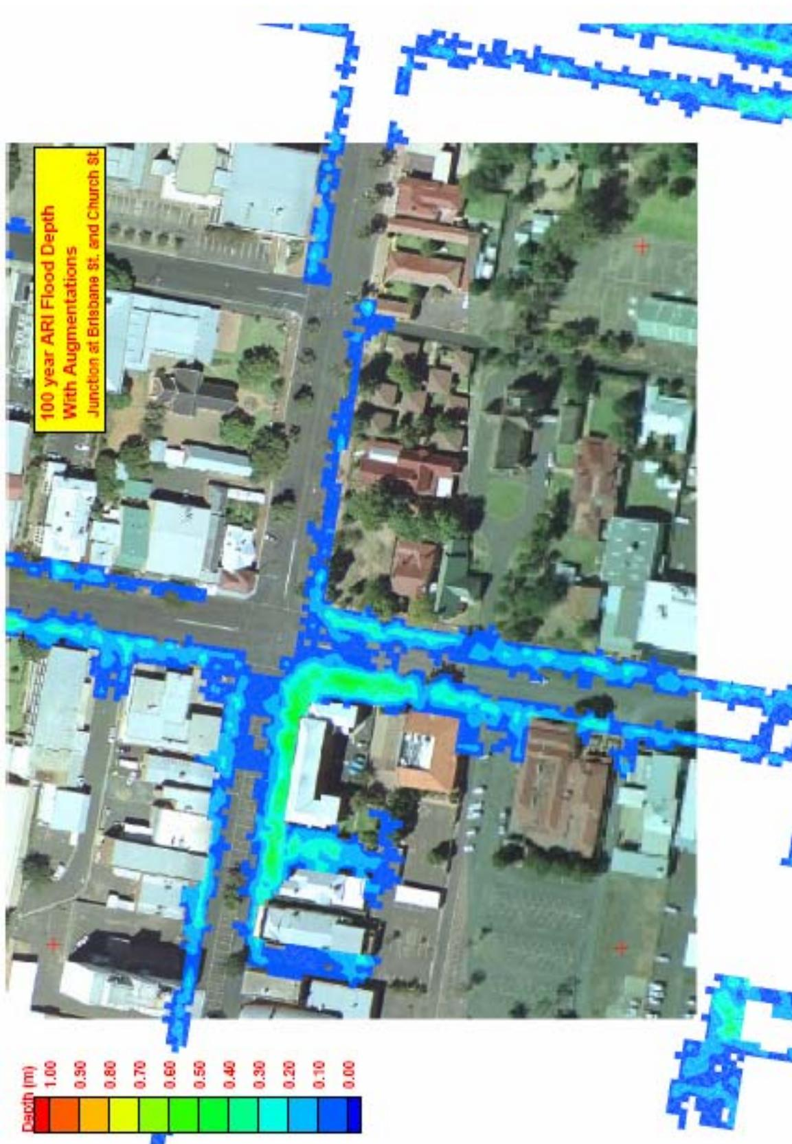
Figure 5 Estimated 100 yr ARI Flood Depths and Extents at Brisbane Street & Church Street Intersection – With Concept Augmentation Works
