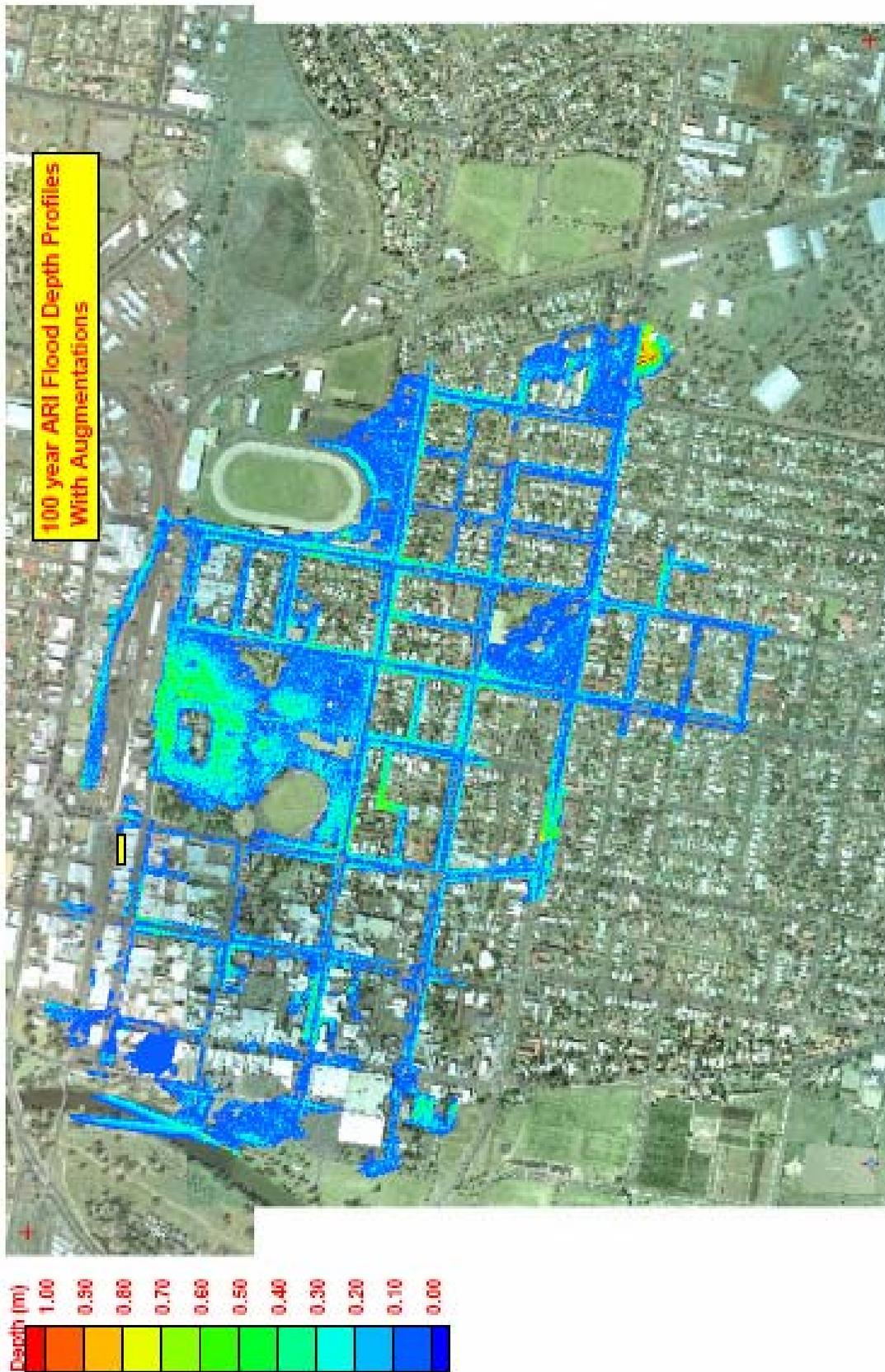
Figure 3 Estimated 100 yr ARI Flood Depths and Extents – With Concept Augmentation Works
