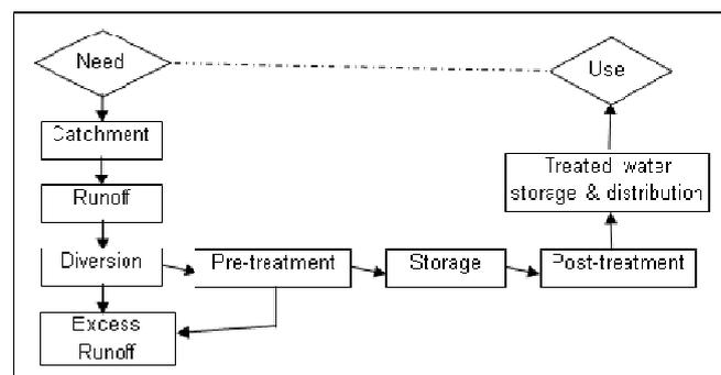
Fig. 1 Generic Stormwater Harvesting Flow Diagram (Source: [15])
