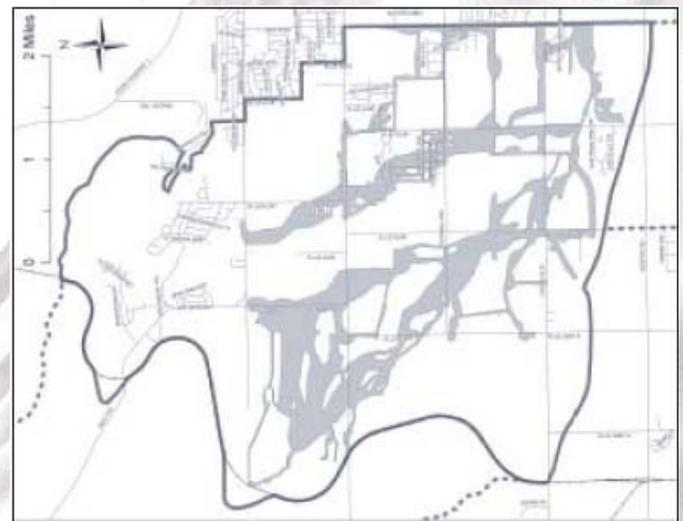
The team also had to account for Billings' existing infrastructure such as culverts, bridges and roadways that could act as dams in the event of a flood, influencing the water's route. These impacts needed to be precisely reflected in the model and were beyond the capabilities of one-dimensional modeling, which assumes water is flowing in one direction. PBS&J's model
